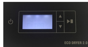
Touch pad controller and display panel
